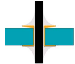
Figure 3. Cross section of solder joint with a lifted pad Example of lifted pad phenomena
