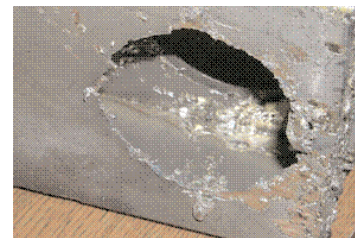
Figure 4. Example of solder pot damaged from Lead Free solders.
