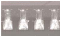
Figure 5. Examples of SnPb versus Pb solder joints.
